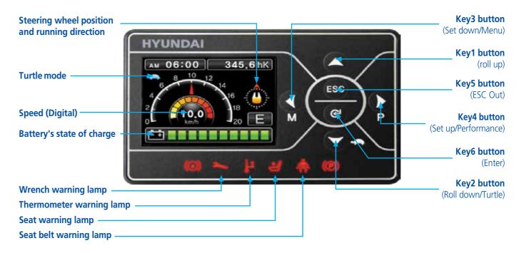
The LCD color monitor with 3.5 inch graphic smart display allows the operator to easily and efficiently control the machine. The monitor provides information about speed & accelerator level, steer angle & travel direction, battery discharge indicator, hour meter & working mode. The operator can select various performance modes to meet all working conditions. It is available multi-languages (maximum 11) for operator.
